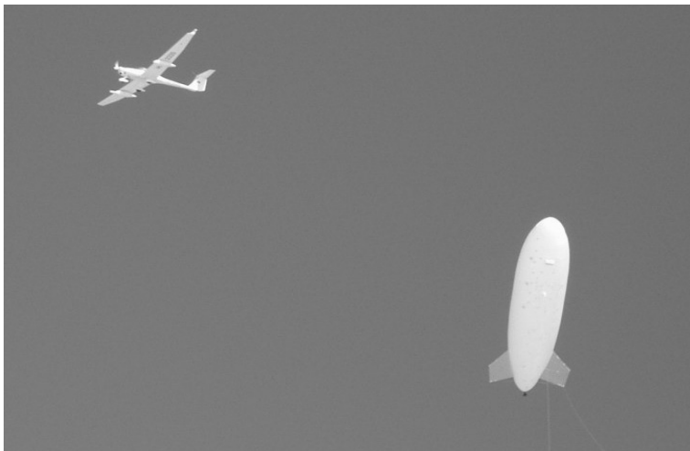
Figure 1: The two measurement platforms of the INNOX-project can be seen on this picture: The research aircraft (type: Dimona) which measured from about 150 to about 2200 m AGL (crest height) and the Balloon (filled with Helium) that rose to about 150 m AGL.
